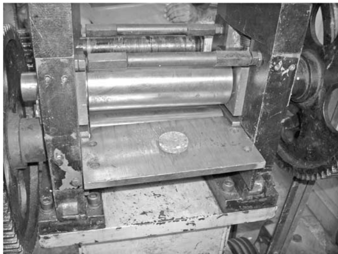
Fig 9: Sintered metal for rolling in 2-high rolling mill
