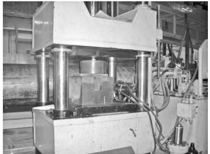
Fig 7: Hydraulically operated compaction press
