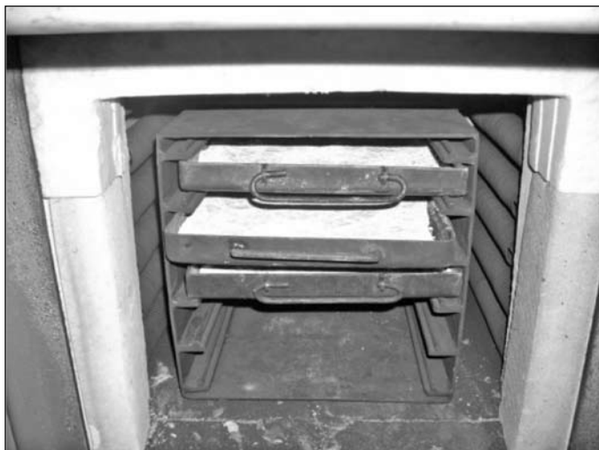
Fig 2: Calcination of thorium oxide powder
