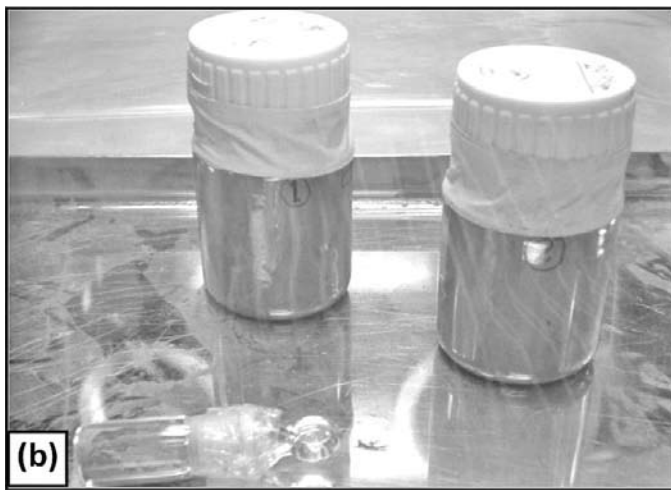
Fig 6: (a) Wet thorium powder and (b) Thorium powder after vacuum drying
